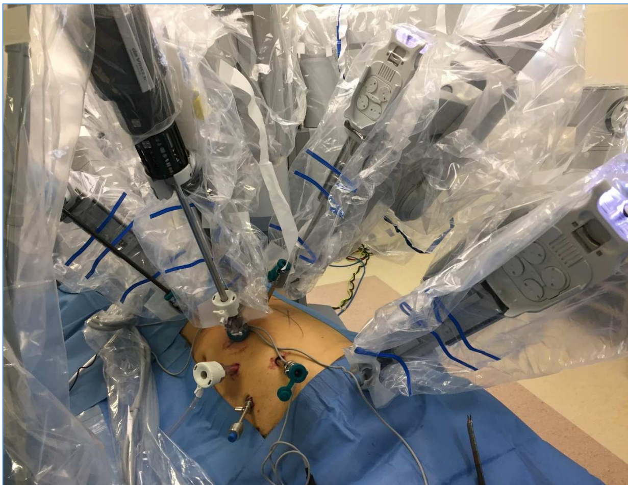
Figure 5.14.2. Robot position after redocking for the distal ureterectomy with the use of the third arm.
