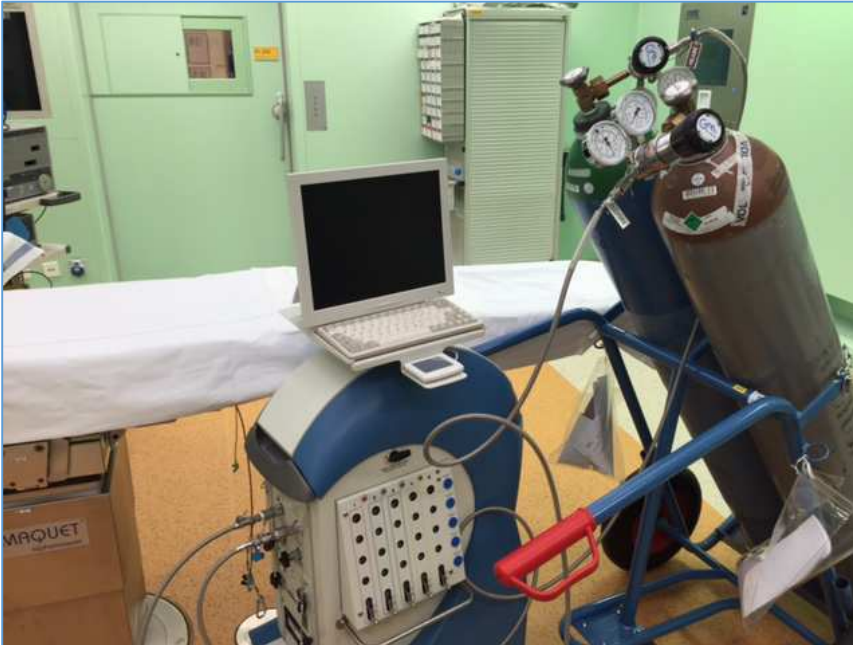
Figure 5.4.2. Helium and argon bottles connected to the cryo-device in the operating room
