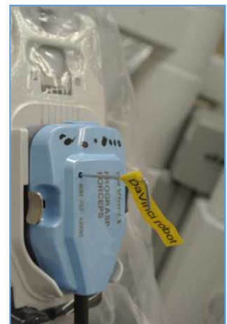
Figure 2.1.6. Key for mechanically opening the robotic grasper
